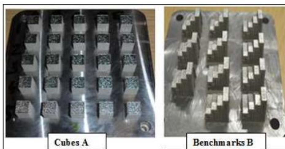
Figure 5 The SLM 125 was used to make cubes as well as benchmarks
